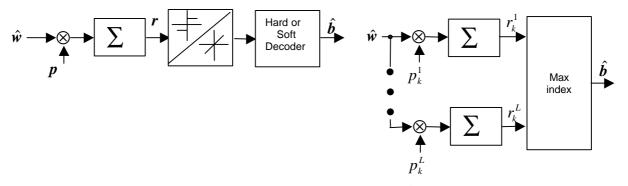
Figure 3. Optimal hard/soft decoder for ECC (a) and for M-ary modulation (b):  $p_k^i$  is a set of orthogonal functions used for the allocation of the *k*-th bit (block) of message, for the *L* orthogonal sequences chosen according to the key.
