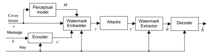
Figure 1. Communication formulation of a watermarking system.
