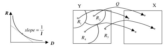
**Figure 5**. Rate-Distortion curve for some coder with the corresponding operational point.
