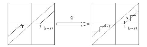
Figure 7. Approximation of the soft-shrinkage function by quantization with zero-zone.
